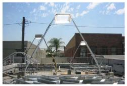
Rooftop solar concentrator eliminates 95% of the silicon-based PV material required to produce a given amount of energy
