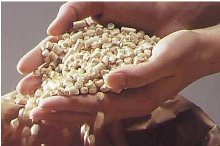
Figure 13: Typical wood pellets may be 6-7 mm in diameter, 8-10% moisture by weight, and have density of about 600 \text{ kg/m}^3 of the moist wood material (Theka and Obernbergera, 2004). This photograph is from www.woodpellets.org .
